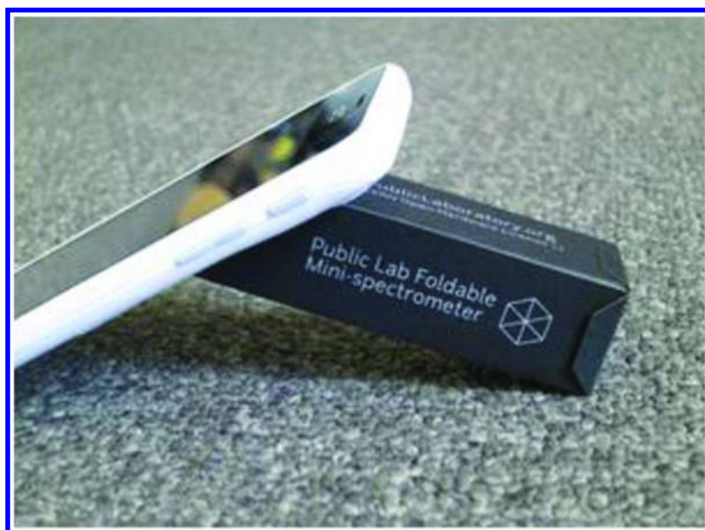
Figure 2. PublicLab smartphone spectrophotometer.
